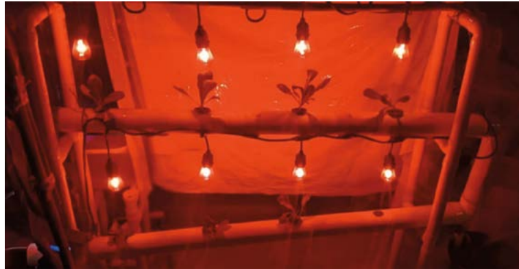
Figure 6. NFT system with the artificial illumination turned on. The figure displays a system designed for eight plants.
